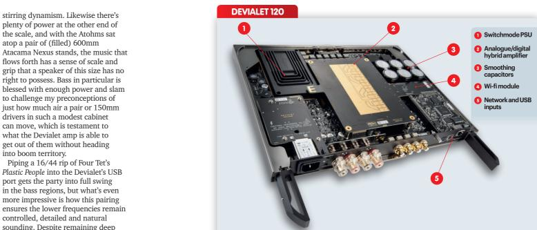
Tested with the latest v7.1 firmware nstalled, this 120 ADH amplifier met its 120W/6ohm specification with a full 2x75W/8ohm, doubling to 2x 150W/4ohm - this power achieved with a peak level (OdBFs) digital input and the volume control set at +0.5dB
